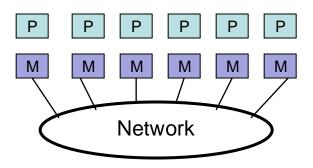
Distributed memory: each processor has its own local memory. Must do message passing to exchange data between processors. cc-NUMA enables larger number of processors and shared memory address space than SMPs; still easy to program, but harder and more expensive to build. (example: Clusters)
