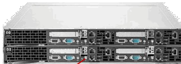
Tested 1/4 server, 8/8 cores, Nehalem-EP @ 2.93 GHz, 24 GB DDR3; peak Tflop/s = 0.2 single, 0.1 double
