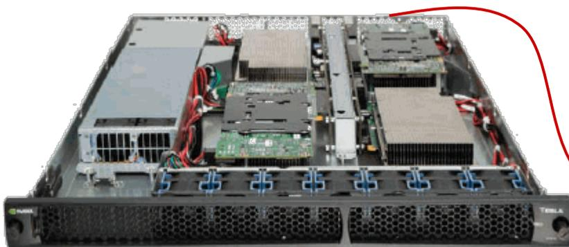
Tested 1/4 T10 @ 1.44 GHz, 4 GB GDDR3; peak Tflop/s = 1.0 single, 0.1 double
