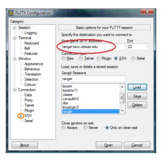
4. Open the SSH menu, in orange on the left of the picture above. Choose X11 settings, shown on the left below, to find the button to "Enable X11 forwarding."
