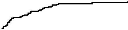
Fig. 8.16 Tiny jumps: Barkhausen noise. Blowing up a small portion of Fig. 8.15, we see that the magnetization is growing in a series of sharp jumps, or avalanches.
